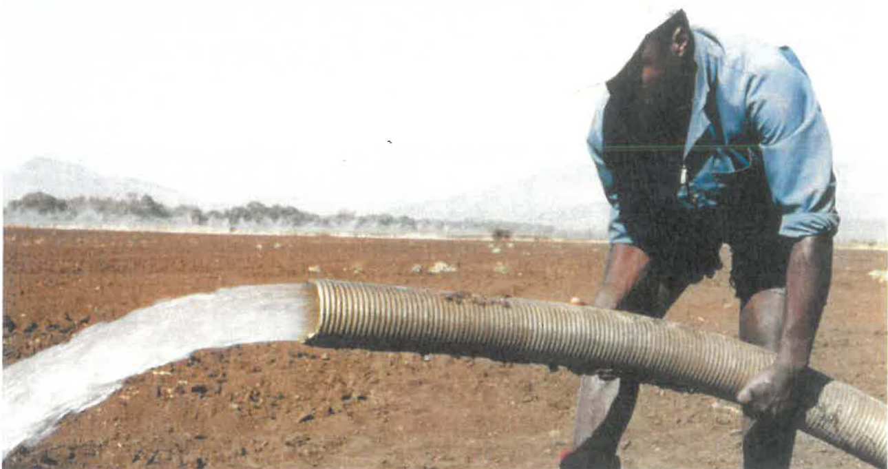
Plate 2. Discharge of 16 l/s produced by a borehole tapping alluvial sediments building the primary aquifer of the Crocodile River valley floodplain. Tree line marks the river channel. (Photo: PJ Hobbs)
