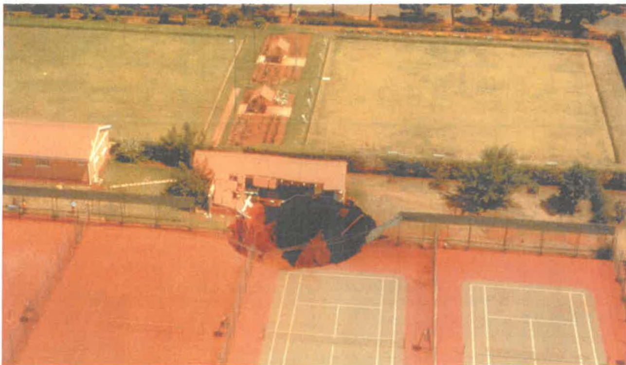
Plate 4 Catastrophic damage to surface structures caused by a sinkhole. (Photo: Council for Geoscience)
